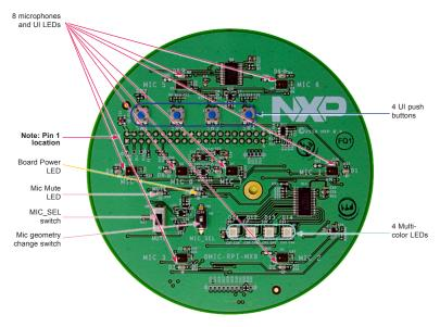
Figure 2: Front View of the 8MIC Board
