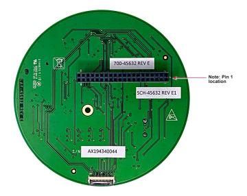
Figure 2: Back View of the 8MIC Board
